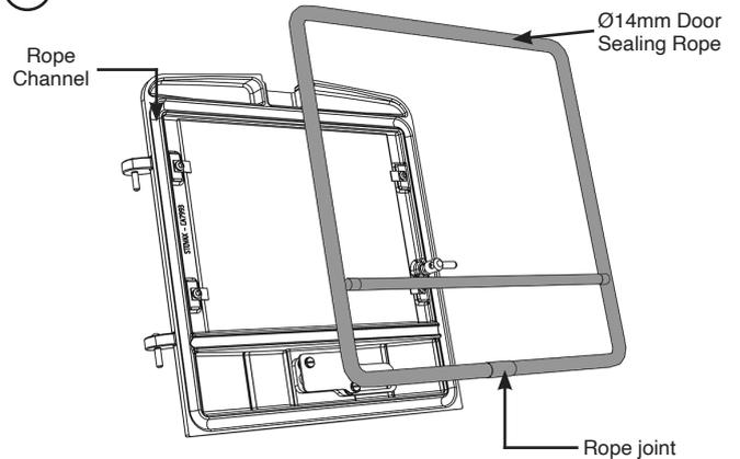
Remove the old rope and scrape old glue from the locating groove.
