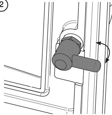
Wind clockwise to tighten door gap
