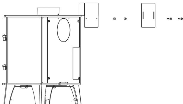
Align the Heat Shield on the slots to cover the gap between the Twin Wall and the Top Plate. The overlap must be at least 10mm.
