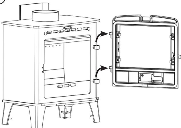
Lay the door face down on a soft flat surface, to protect the paintwork and glass.
