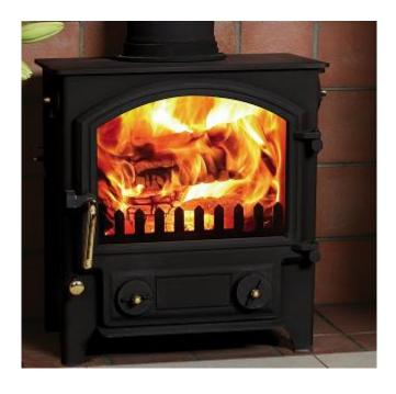
The Little Thurlow Smoke Control Eco stove has a nominal heat output of 5kW., and a weight of 61 kg. The flue gas mass flow is 4.3 g/s for wood logs, 3.7 g/s for solid fuel. The mean flue gas temperature directly downstream of the flue spigot at nominal heat output is 281 degrees C (wood) 276 degrees C (solid fuel). The stove is designed as a closed appliance and is capable of intermittent operation. Tested Net efficiency 79.0% (wood), 80.2% (solid fuel).
