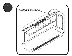
Make sure that your fireplace is plugged in and the mains power is on. Then turn on your fireplace by pressing the ON/OFF switch to the 'ON' position.
