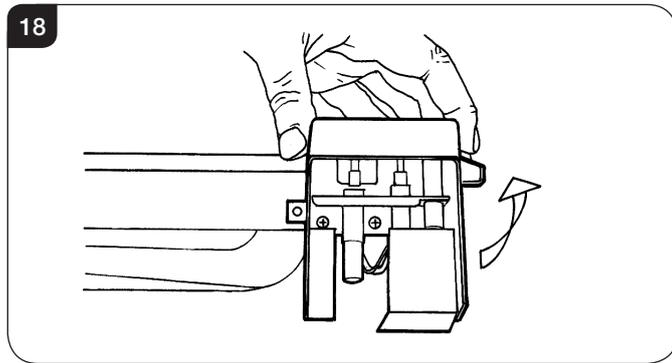
5.3 Remove the 2 screws securing the pilot assembly, see Diagram 19, Arrow C.
