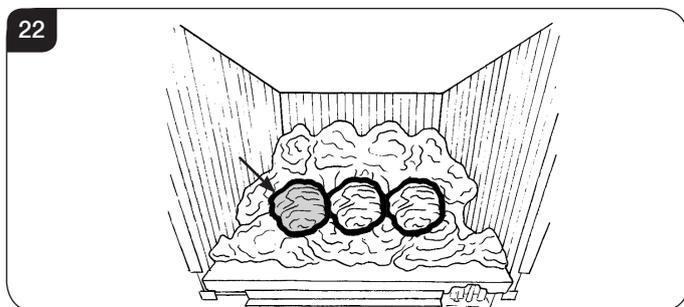
5.18 Place a small coal directly behind the first large coal, and rest it on the flame baffle, see Diagram 23.
