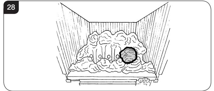
6.16 Place a second single large coal in the middle dent of the front coal resting against the flame baffle, see Diagram 29.
