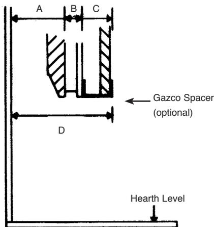
The appliance can also be fitted into a metal flue box with a 5" (125mm) diameter flexible liner. In this installation a 1" (25mm) rebated fire surround must be used. Refer to Diagram 3, Pre Fab Metal Box for dimensions.
