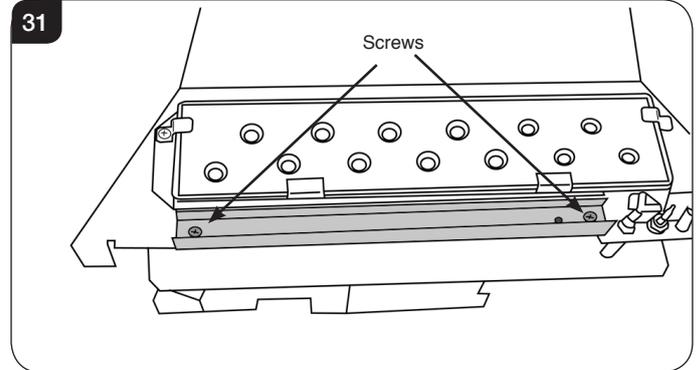
6.26 Undo the 2 screws securing the bracket to the bottom of the burner unit, see Diagram 32.
