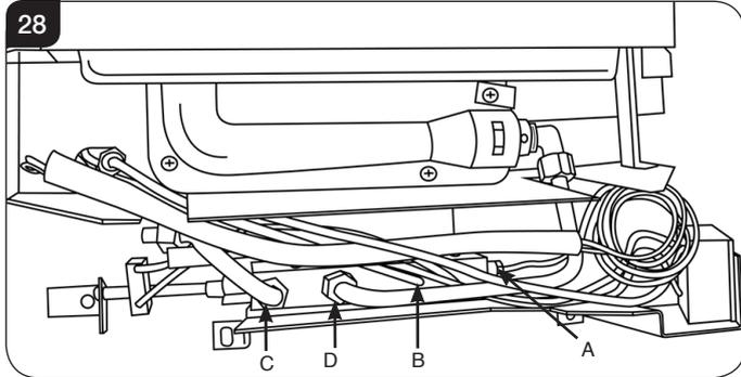
6.19 Undo the pilot pipe from the gas valve, see Diagram 28, Arrow B.
