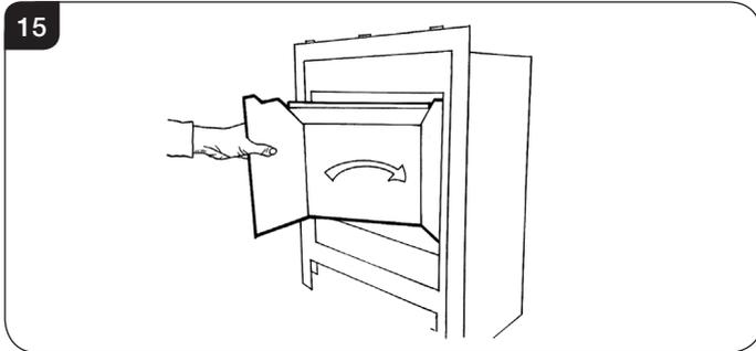
5.2 Check that the panel is sitting behind the rear ledge of the burner, see Diagram 16.
