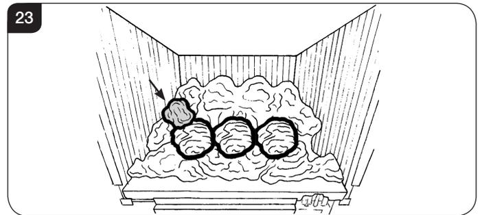
5.19 Place two of the remaining small coals in the spaces next to the first. The final small coal sits at the front right next to the large coals, see Diagram 24.
