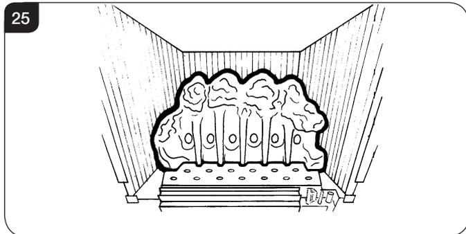
6.13 Place the front coal centrally in the channel at the front of the tray. The relationship between the front coal and the flame baffle is shown in Diagram 26.
