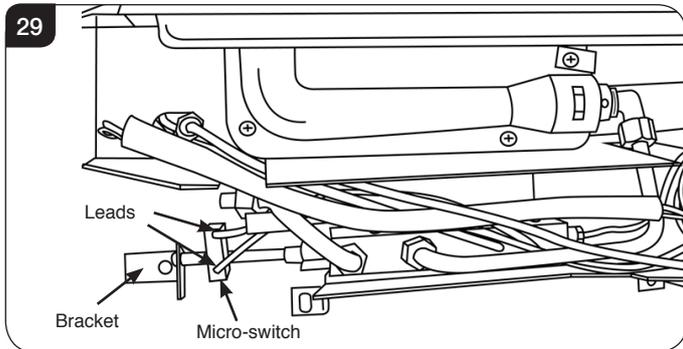
6.23 Undo the screw from the end of the spindle and remove the bracket, see Diagram 29. Ensure bracket is replaced during reassembly.
