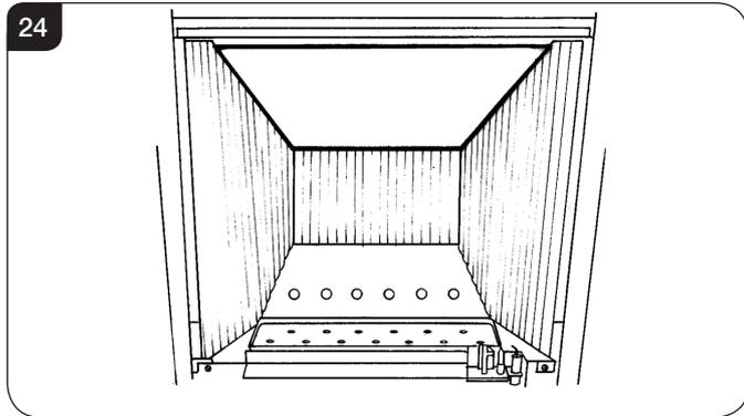
6.12 Position the flame baffle centrally on the tray and ensure the stepped lower edge engages against the rear edge of the burner skin, see Diagram 25.
