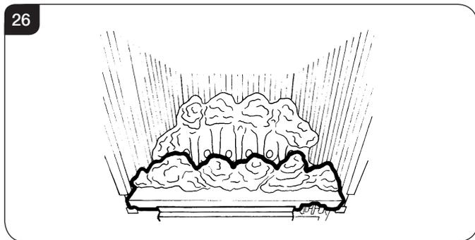
6.14 There are three sizes of coal used: 3 x Large, 4 x Small and 1 x Half Moon shaped. For identification, see Diagram 27.
