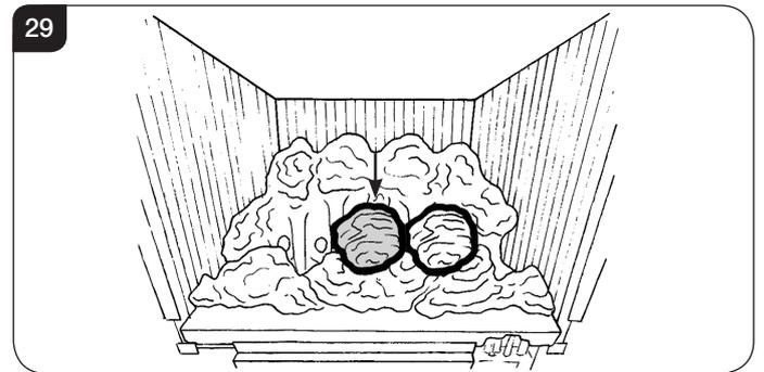
6.17 Place the third large coal next to the first middle coal and against the flame baffle, Diagram 30.
