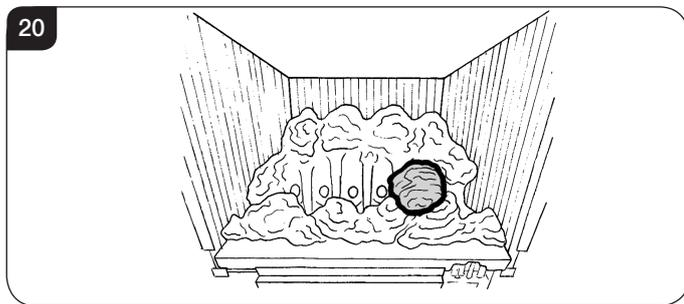
5.16 Place a second single large coal in the middle dent of the front coal resting against the flame baffle, see Diagram 21.
