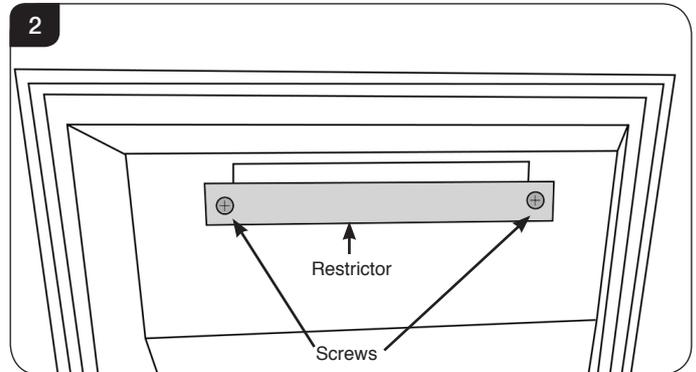
This is fitted from outside the appliance across the outlet at the top of the box with 2 screws provided.
