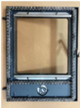
**FIRE DOOR:** Remove the 4 or 6 stainless steel screws retaining the double glazed glass panel. This panel is two pieces of glass with a 2mm x 10mm seal between them. Replace the 2mm x 10mm seal if necessary. Position replacement glass and fit retaining channels, tighten screws just enough to pinch the glass. Overtightening can result in the glass cracking.
