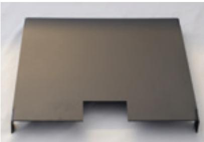
**To fit:** Slide in at the base of the stove prior to installation. It needs to slide in from the **rear**. The edge with the cut-out should slide in first, resting at the front of the stove. The folded legs of the heat shield will sit on the tabs for the leveling screws, (these are small square tabs with a hole in the centre).
