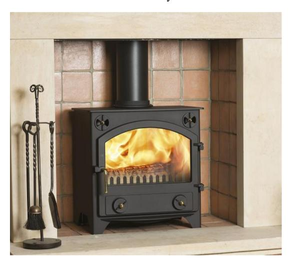
The Bransdale SC ECO stove has a nominal heat output of 8kW and a weight of 100 kg. The flue gas mass flow is 5.4g/s for mineral fuel and 6.7g/s for wood logs. The mean flue gas temperature directly downstream of the flue spigot at nominal heat output is 316 degrees C (wood) 342 degrees C (solid fuel). The stove is designed as a closed appliance and is capable of intermittent operation. Tested Net efficiency 77.1% (wood) and 77.8% (solid fuel).
